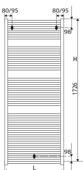
Bracket measurements are 80 mm (straight) and 95 mm (curved) from either side of the towel rail and 98 mm from the bottom.
